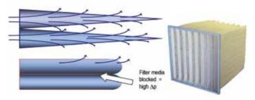
Figure 6: Schematic air flow in correctly designed and poor quality bag filter
