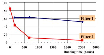
Figure 3: Increase of efficiency due to electrostatic charge
