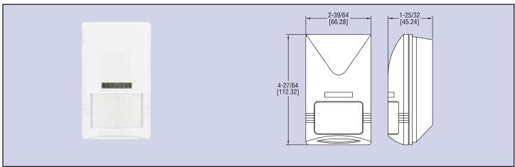
The Model OSW-100 Wall Mount Occupancy Sensor is an infrared sensor designed to automatically control a HVAC ventilation system. A unique dual delay processor eliminates false triggers due to short-term occupancies. The Model OSW-100 has a wide 110° viewing angle to capture movement up to 49.2 ft (15 m) away.
