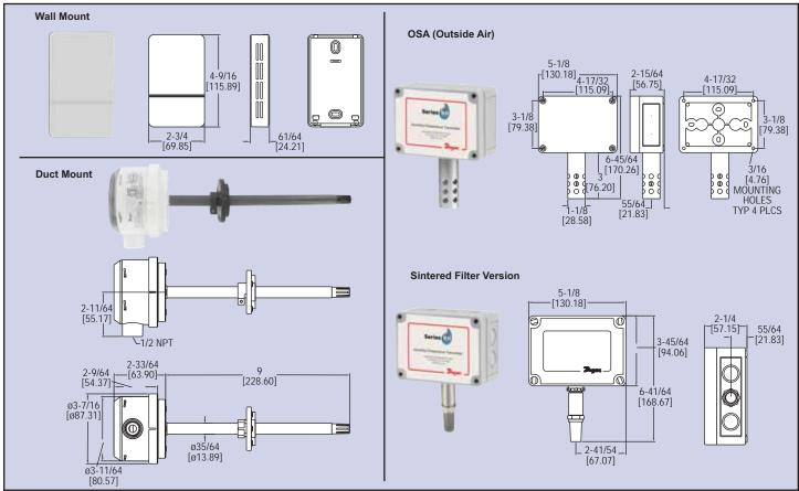
Demanding humidity/temperature applications require the Series RH/RHL Transmitter which offers high accuracy, long term stability, and reliable operation. The Series RH/RHL is designed for monitoring and controlling humidity or both humidity and temperature in building energy management systems, HVAC, commercial, residential, clean rooms, museums, climate chambers, and other space monitoring applications.
